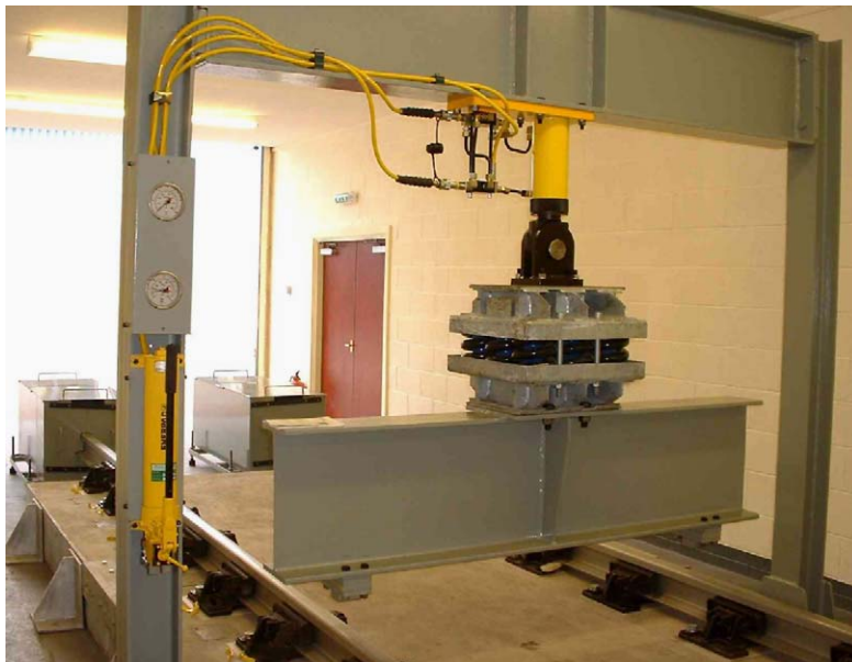
Fig. 1. A photograph of the CONVURT test rig.
